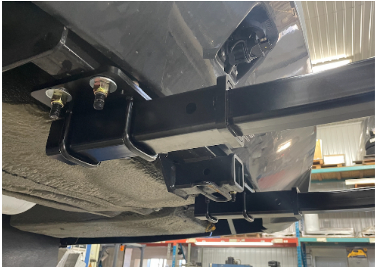
Step 2: Take the other 2 x U-bolts and place around end of receiver, insert them through the plate provided and secure them tightly with washer/nuts provided. Then secure plate to the U-bolts you previously put around your receiver frame with the washer/nuts provided
